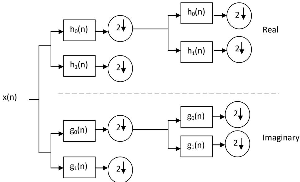
Fig. 1 Filter bank of Two Level DT-CWT
