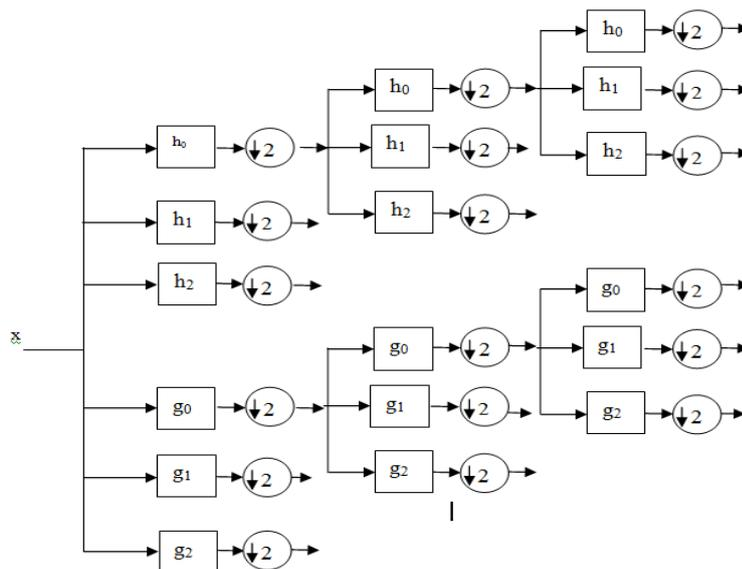
Fig. 2 Iterated filter bank for the DD-DT-DWT
