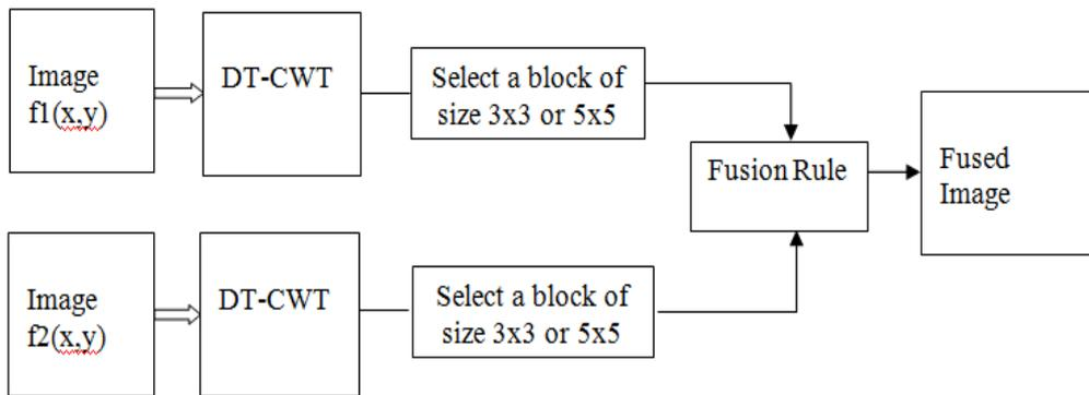
Fig. 3 Image fusion block diagram
